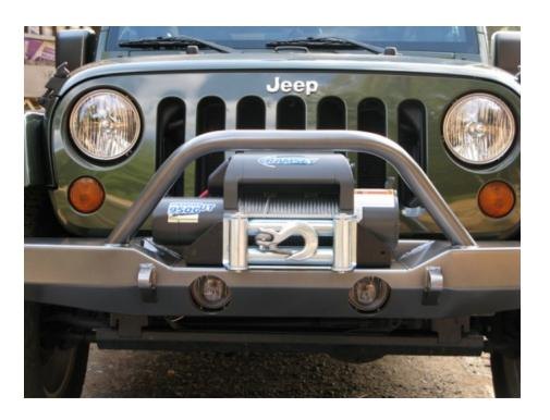
Tighten all bolts and check for proper fog light pattern, adjust if necessary.
