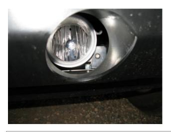
Once light is in the bumper it will mount to the bumper using two 1/4" SS bolts and nuts. Install the button head bolt from the bottom up through the light bracket, align and tighten.
