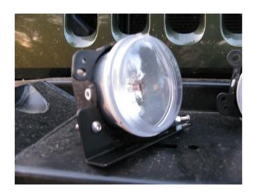
Mount the supplied steel mounting bracket to the light using 1/4" SS bolt and nut.
